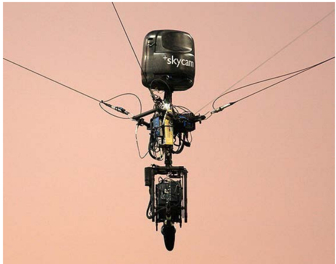
Figure 2 SkyCam: a commercialized suspended cable robot
